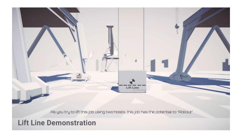
When your lift points are below the center of gravity it is important to add base hitched to prevent rollout as the example above demonstrates.
