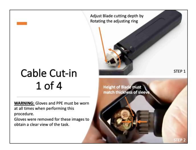
Adjust the cutting blade depth to ensure it does not cut all the way through the insulation and into the conductor itself. Ensure that you wear the proper gloves and other PPE to prevent injury. Gloves are removed in this and the next few slides to provide a better picture of the tools and conductors.
