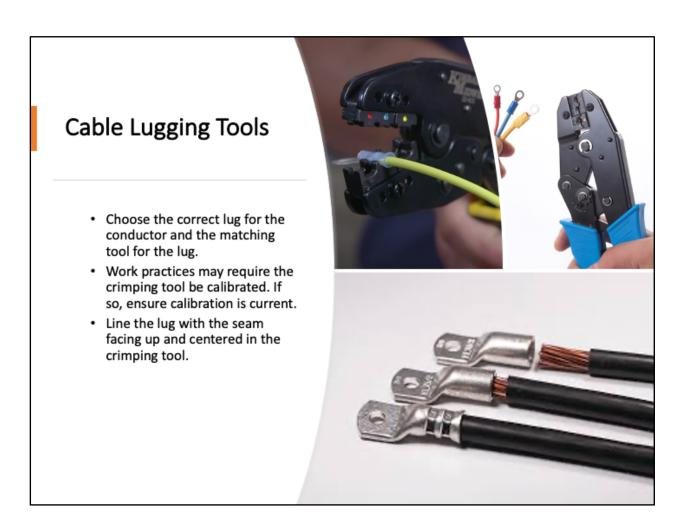
You must be careful to use the correct lug for the conductor and the matching size nest on the crimping tool.
