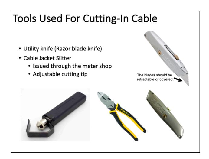
Basic cable cutting requires tools to remove the cable outer jacket, remove the insulation, and access the conductor.
