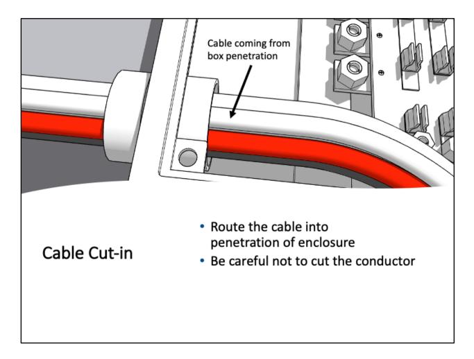
Cable Cut-in refers to bringing a cable into or through an enclosure. First, mark the cable in the location where the jacket must be cut, usually about 1/8 inch from the penetration point.
