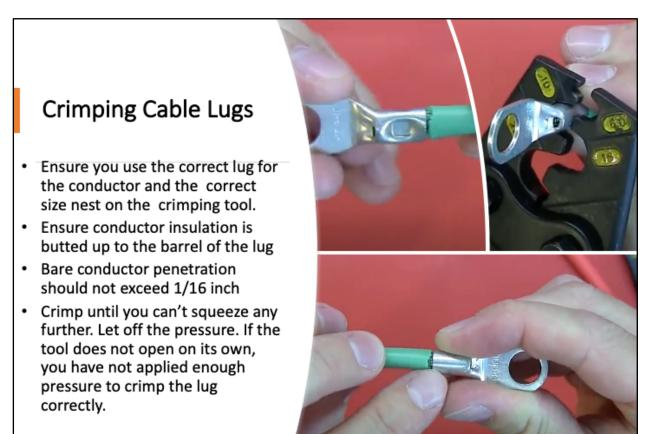
Ensure you have the correct lug for the conductor and the correct crimping tool. Remember, some crimping tools must be calibrated. If required, make sure calibration is current before using the tool.
