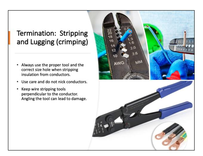
Always use the proper tool when removing conductor insulation. Do not be tempted to save time by using wire cutters or a knife!
